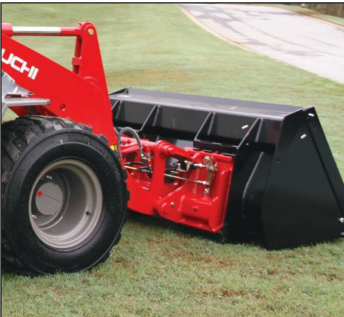
The versatile hydraulically operated skid steer style attachment coupler is easily controlled from the operator's seat.
