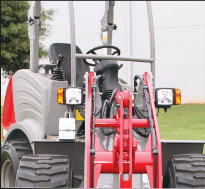
Heavy duty loader arms, oversized pins and self-aligning cylinder bushings deliver excellent performance and durability for maximum uptime.
