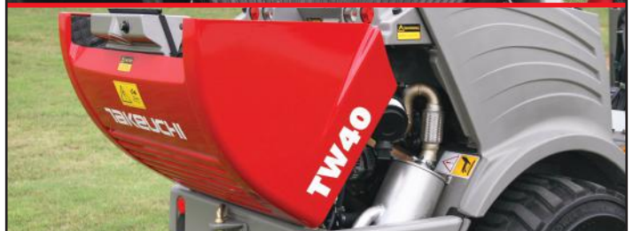
The lockable rear hood provides access to daily inspection points including engine oil dipstick, hydraulic oil sight gauge, air filters and radiator/oil cooler.
